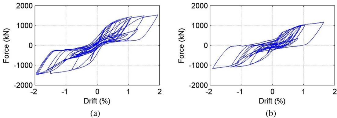
Figure 6: 10/50 force vs. drift response for (a) Specimen FR and (b) Specimen NZ
