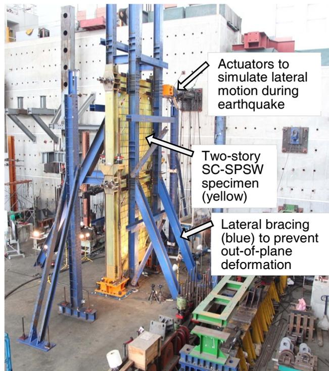
Figure 3: Test setup, shown here for Specimen FR.
