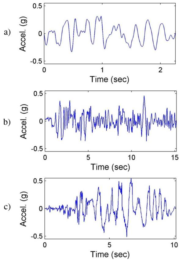
Figure 4: Excitation used for the (a) 50/50, (b) 10/50, and (c) 2/50 pseudo-dynamic tests
