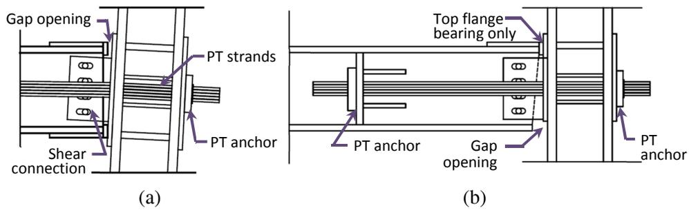
Figure 1: Schematic of (a) Flange Rocking and (b) NewZ-BREAKSS PT connections
