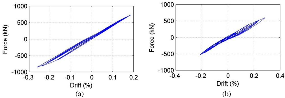
Figure 5: 50/50 force vs. drift response for (a) Specimen FR and (b) Specimen NZ
