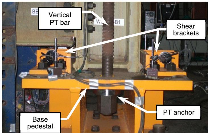
Figure 2: PT column base connection
